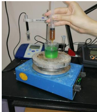
Figure 2. Dripping alginate and ferric oxide mixture into the \text{CaCl}_2 solution
