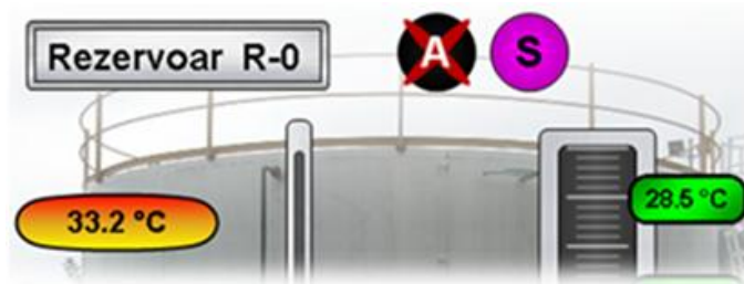
Figure 7. Tank designation, Blocked alarm active simulation sign
