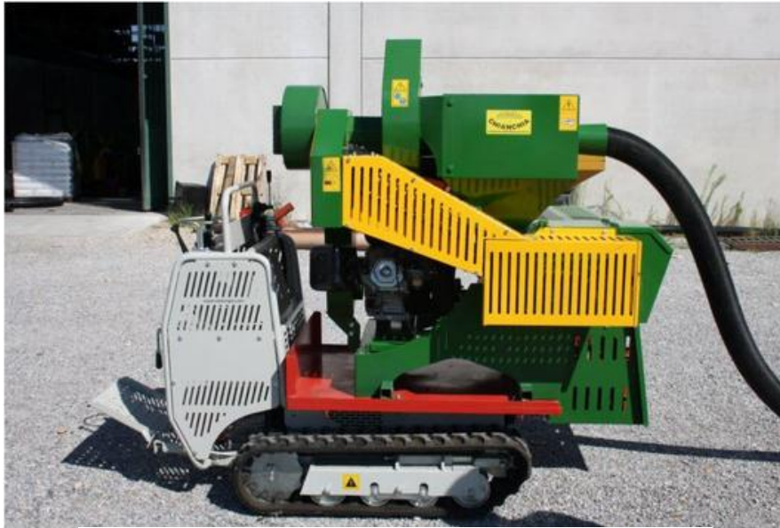
Figure 4. Vacuum suction unit adapted to the crawler digger
