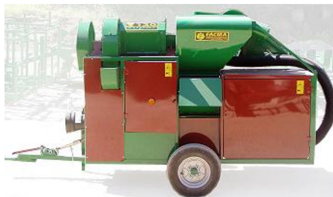
Figure 3. Tractor-adapted vacuum suction unit with grain extraction function
